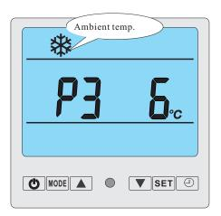
© Under running status ,press "M" 5 seconds to check the current status of the unit!You can check water-in/water out temp,condenser temp and ambient temp,please note no motion on the display for 10s,the LCD will display water-in/water out temp/(under running)or ambient temp.(unit stops)
